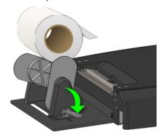
d Insert stock into input slot
