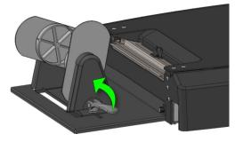
Place roll on fixed holder, slide adjustable holder onto core, lock lever down
