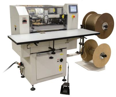
The **BB50H** High Speed Semi-Automatic Binder finishes documents up to 20" wide, with output speeds of up to 1200 books/hour. The **BB50H** automatically finishes pre-punched documents with Wire-O® sizes from 1/4" up to 1", using traditional spools or our patented SnakeSkin™ Wire-O® in 3:1 and 2:1 pitches. Size, pitch and format changes are electronically controlled from the user-friendly touch screen. The **BB50H** can skip bind and an optional calendar hanger feed system is available.
