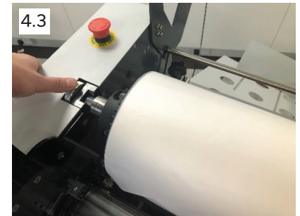
4. Slide film onto the mandrel and centralize (4.1). Replace the core adaptor and tighten. Place the mandrel back onto the system and tighten the mandrel lock (4.3).
