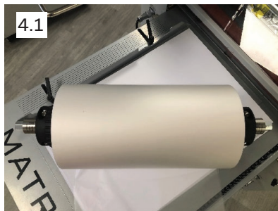
4. Slide film onto the mandrel and centralize (4.1). Replace the core adaptor and tighten. Place the mandrel back onto the system and tighten the mandrel lock (4.3).
