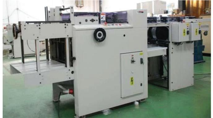
The configuration changeover is very easy and both reception devices can be disconnected. The mechanical device is operated by a handle; the electrical device is driven by an on/off switch. work.
