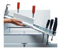
Convenient drop-in tool holder on rear of machine keeps various routine maintenance tools close (including for blade change)
