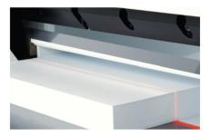
German high speed steel knife with swing cut motion ensures the highest level of cutting accuracy & quality
