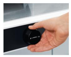
Electronic hand wheel for manual back gauge positioning option
