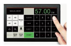
Large 7" touch screen control panel is convenient & easy to use. Set up the back gauge and exact measurements, or recall past jobs with the large memory storage (99 jobs & 99 steps in each job)
