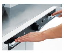
Easy cut blade activation bars require two-hand operation and allow blade & clamp to perform independently
