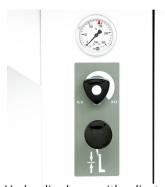
Hydraulic clamp with adjustable pressure from 1,900 to 3,800 psi for use with even fragile prints
