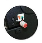
**Depth Margin Control**4 possible settings provide the correct punch margin depth for each wire size.
