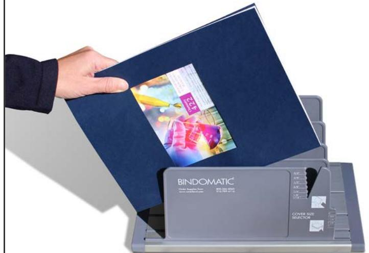
**4** Wait for the machine to signal that the thermal binding process is complete. Remove the bound books from the heating plate. Allow the finished books to rest spine-side-down in the cooling rack for two minutes before opening.
