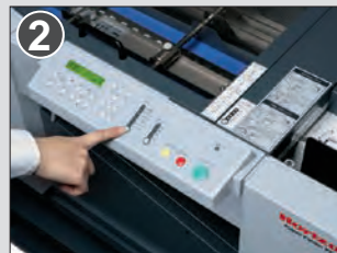
2 Select sheet size and fold pattern.
