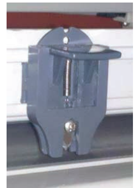
Cross cutter permits simple cutoff as the laminated material exits the rear of the machine
