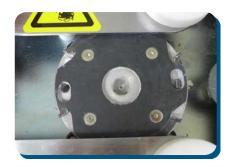
New spine roughening with 1 notching blade and 6 milling blades provides better glue penetration while applying the glue onto the book spine.
