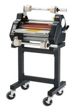
**Tamerica's VersaLam 1300** is a 13" wide roll laminator that can be used with film up to 10mil thick. The **VersaLam 1300** includes variable speed and temperature control for laminating a variety of projects, as well as the ability to turn off the heat to the bottom roller for one-sided lamination. The heated rollers are manufactured of top-grade silicon rubber that help to ensure bubble and scratch-free lamination.
